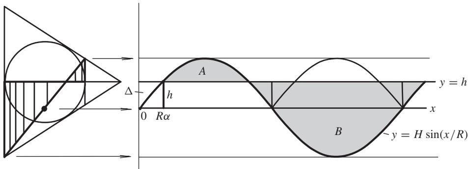
**Figure 12.** Lateral surface area  $S_2$  is twice the sum  $A + B$  of the areas of the shaded sinusoidal regions.
