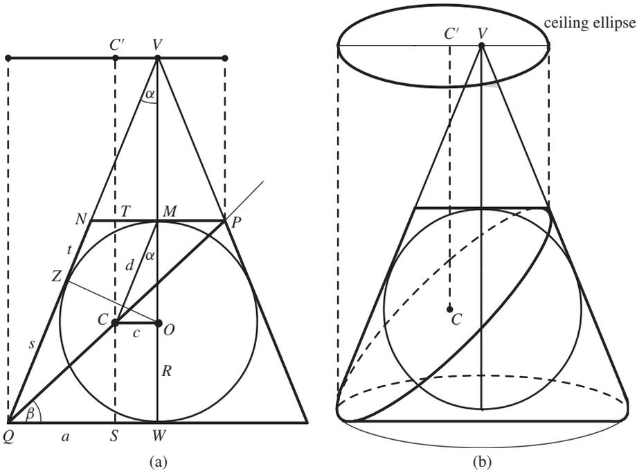
**Figure 9.** (a) Vertical cross section of the intersection of cone and cylinder circumscribing the same insphere; (b) the ceiling ellipse is the vertical projection of the slanted ellipse onto a horizontal plane.
