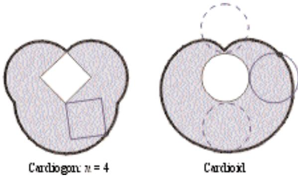
**Figure 3.** A cardiogon traced by the vertex of an  $n$ -gon rolling outside an  $n$ -gon. The cardiogon becomes a cardioid as  $n \rightarrow \infty$ .
