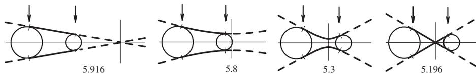
**Figure 21.** The hyperbola degenerates to a pair of lines when  $c = \sqrt{d^2 - (r_1 - r_2)^2}$ . As  $c$  decreases further the hyperbola flips and opens up and down instead of right and left, until the next degeneration occurs at  $c = \sqrt{d^2 - (r_1 + r_2)^2}$ . This interval for  $c$  represents abnormal configurations not realizable on a cone, but requiring a twisted cylinder.
