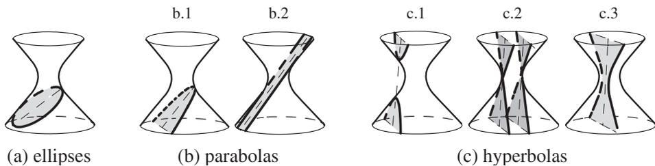
Figure 2. Intersections of a twisted cylinder with an inclined plane.
