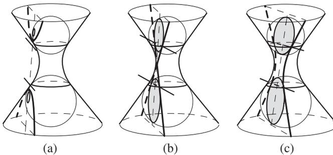
**Figure 14.** (a) Hyperbola. Translating the cutting plane in (a) produces a degenerate hyperbola (b). Further translation leads to the abnormal configuration in (c).
