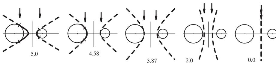
**Figure 22.** For  $c < \sqrt{d^2 - (r_1 + r_2)^2}$  the hyperbola flips back with each branch tangent to one of the disks, until  $c < \sqrt{(d - r_1)^2 - r_2^2}$ , when both disks detach. As  $c$  approaches 0, both branches tend to one vertical line, on which the lengths of the tangents to the two disks are equal:  $t_1 = t_2$ .
