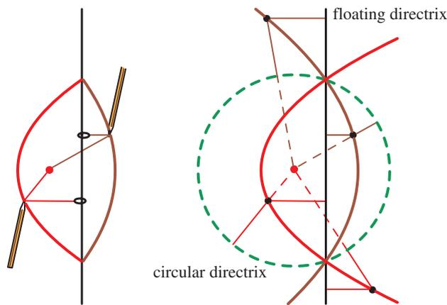
**Figure 12** (a) String construction that gives two confocal parabolas, one on either side of the fixed line. (b) Justification of construction, using the common circular directrix of the two parabolas, with the corresponding floating directrix.
