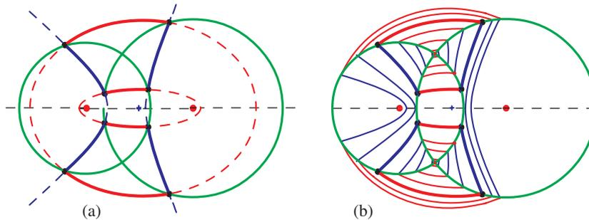
**Figure 4** (a) A curvilinear trapezoid and its mirror image, each traced by one continuous motion of the two-tube string mechanism. (b) A family of trapezoids obtained by varying the length of the portion of the string outside the tubes.
