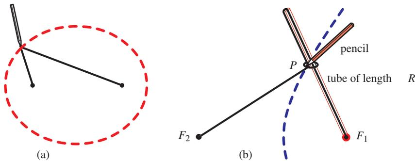
**Figure 1** (a) String construction for the ellipse. (b) New mechanism for tracing a hyperbola. The pencil pushes inward along the outer edge of the tube.
