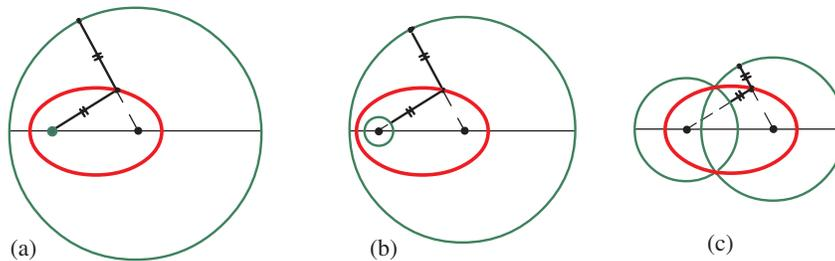
**Figure 6** An ellipse and three pairs of its circular directrices. In (a),  $R_1 = 0$  and  $R_2 = f_1 + f_2$ . In (b) and (c),  $R_1 > 0$  and  $R_2 = f_1 + f_2 - R_1$ . For each  $P$  on the ellipse, the shortest distances  $d_1$  and  $d_2$  to the focal circles are equal.
